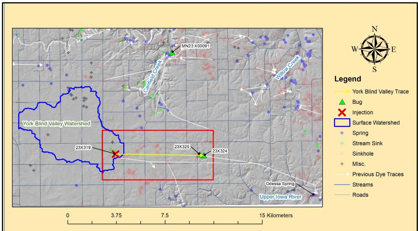
**Figure 5.** 2017 York Blind Valley trace study area. Dye input points, monitoring points, white dye vectors from previous traces in the study area. The rectangle outlined in red is the extent of Figure 6.
