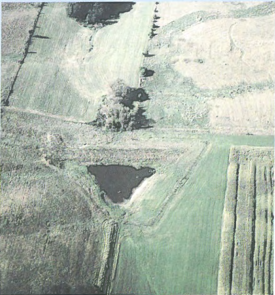
Sediment retention ponds (above) and contour farming (right) were two structural practices used to reduce sediment delivery to Bigalk Creek.
