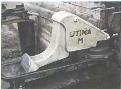
A nose pump (left) is used by cattle (right) as an alternative to giving livestock direct access to a stream.
