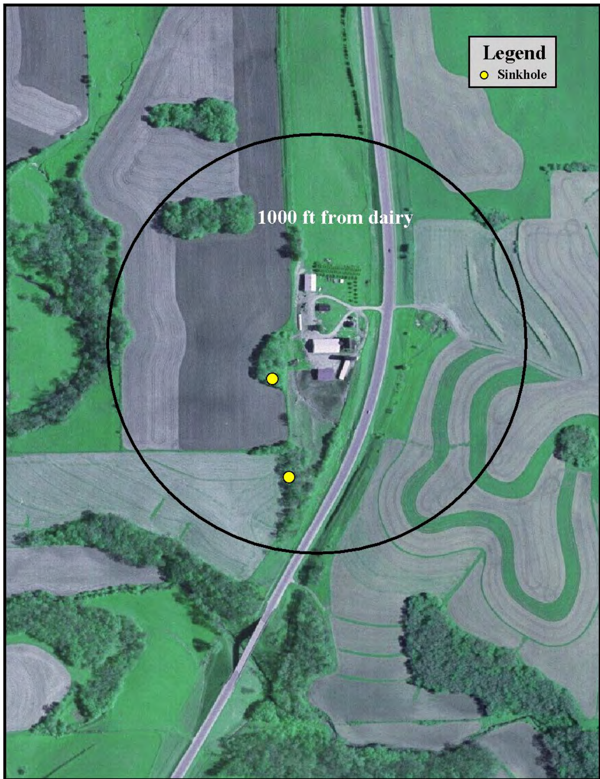
Figure 9-1. Color infrared photo of the Enyart Farm showing sinkholes.
