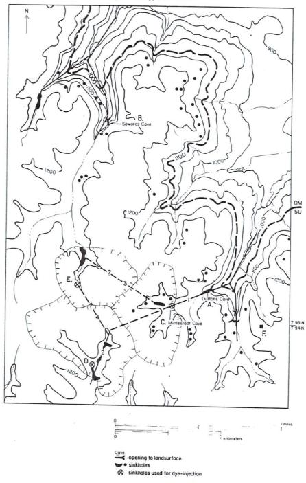
Figure 17. Fayette County dye-tracing study area, showing known (heavy solid lines) and inferred (dashed) linear conduits in area.
