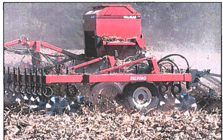
Coulter Harrow (vertical tillage tool) Seeding - air delivery seeder on a coulters harrow in heavy crop residue
