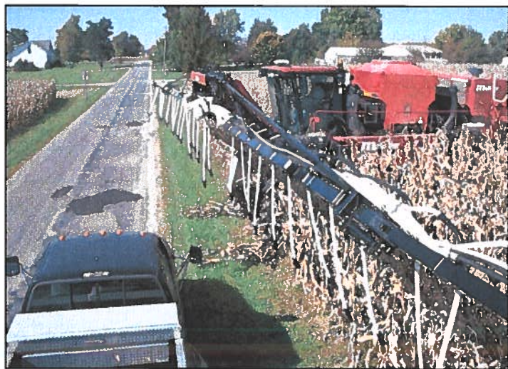
High-Clearance Sprayer, converted to air seed cover crops (photo courtesy of Mike Shuter)
