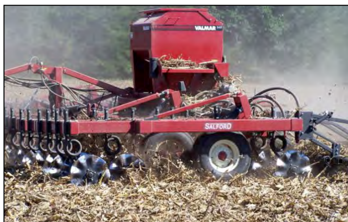
Coultter Harrow (vertical tillage tool) Seeding - air delivery seeder on a coultter harrow in heavy crop residue
