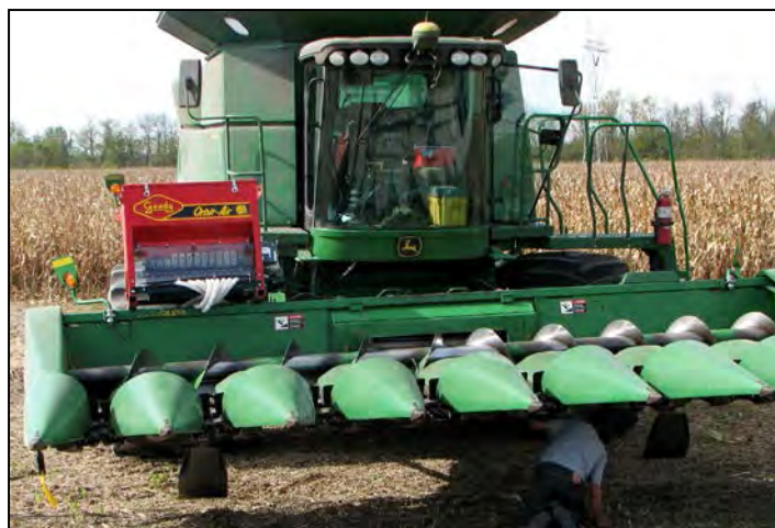
Air seeder mounted to corn head (photo by Ray McCormick)
